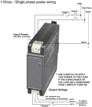
Figure 4.2— Wiring for 115Vac - Single Phase
